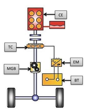
Fig. 1. Architecture of Parallel Hybrid Electric Vehicle
