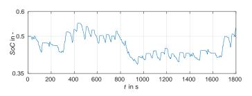
Fig. 7. State of battery charge SoC for FTP.
