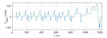
Fig. 2. Torque of manual gearbox  $T_{MGB}$  for NEDC.
