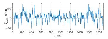
Fig. 5. Torque of manual gearbox  $T_{MGB}$  for FTP.
