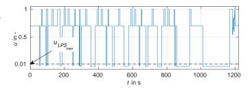
Fig. 3. Torque-split ratio u for NEDC.
