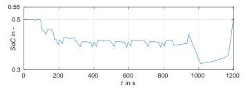
Fig. 4. State of battery charge SoC for NEDC.
